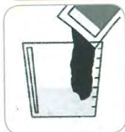
Mix mortar seal with mortar and water
